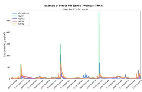
This plot shows examples of subhourly (1-min) indoor PM<sub>2.5</sub> levels that are characteristic of indoor sources or activities that contribute to higher indoor air quality. These spikes coincide with indoor BC spikes. Outdoor PM<sub>2.5</sub> levels are not collected at the sub hourly level.
