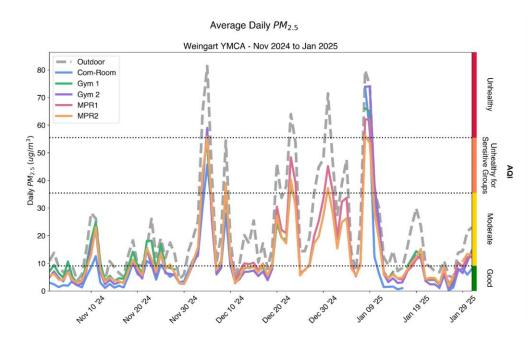
This plot shows average daily PM<sub>2.5</sub> levels across time for both the indoor (solid color lines) and outdoor (dashed grey lines) monitors from the beginning of November 2024 to the end of January 2025. The Air Quality Index (AQI) categories coinciding with PM<sub>2.5</sub> concentrations are shown on the right with bounds shown across the plot in dashed black lines, helping to provide health context. Any gaps in the data are due to issues in power or WiFi/cellular connectivity.
